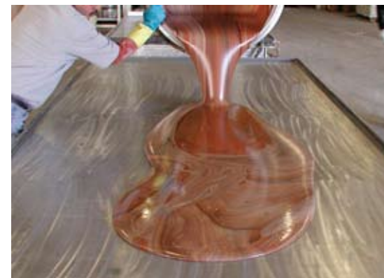
Figure 7: Pour matrix onto table. Spread/ swirl with paddle to enhance look as desired.
